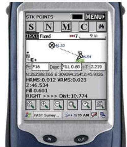
Fast Survey on a ProMark 3 RTK
