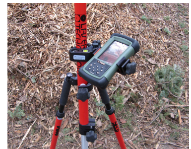
Recon 400X Pocket PC Mounted on a Range pole With Bipod legs
