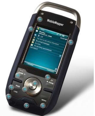
Mobile Mapper 6 ( 2-5 meter accuracy) (1-2 meters with post processing)
