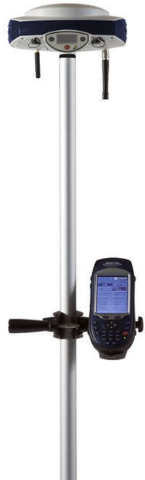
ProMark 500 GPS Unit Set up as a Rover
